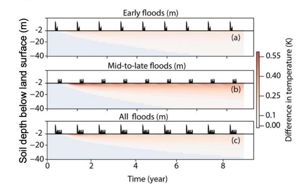
5. Timing of floods is an important factor controlling active layer thickness (ALT). Mid-late summer floods are more likely to cause a deeper ALT, particularly in the first year.
