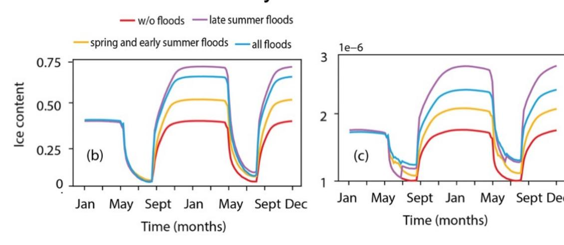
3. Floods cause a soil surface cooling effect due to the increase of latent heat of thawing and evaporation of the wetter soil and deep soil warming effect due to heat penetration
