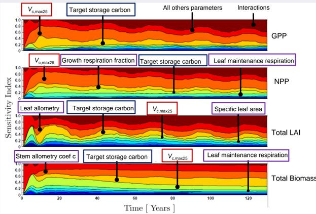
(3) Sensitivity analysis of 66 input parameters into FATES<sup>3</sup>
