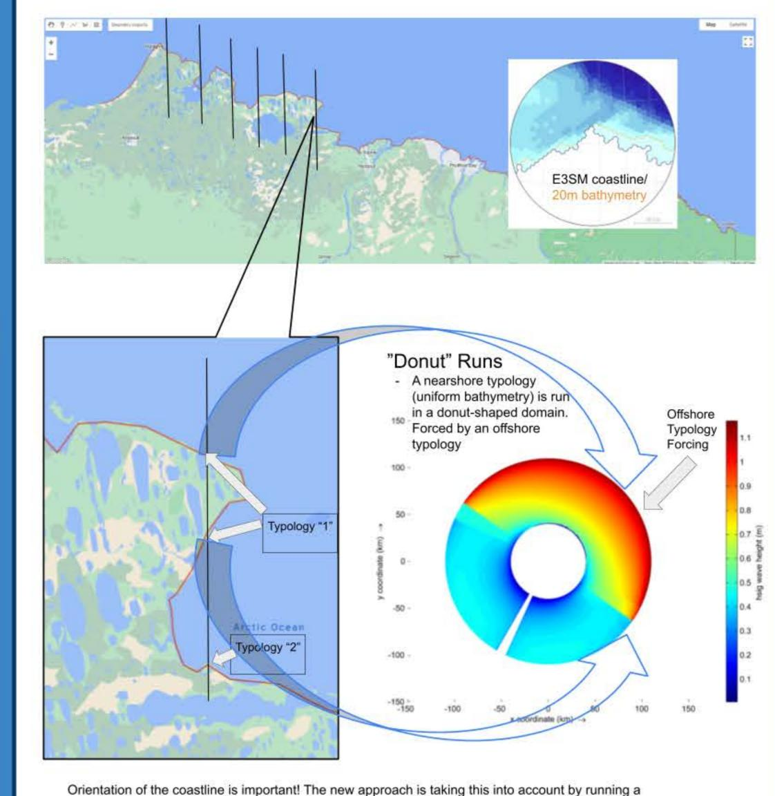
nearshore typology with uniform bathymetry forced by an offshore typology in a circular domain.
