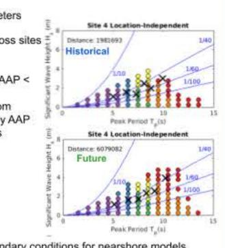
Reduced number of simulations (down from order 10<sup>4</sup> – 10<sup>5</sup> to order 10) needed to assess nearshore oceanographic environments and hence characterize coastal processes (e.g., erosion, flooding, or sediment transport)
