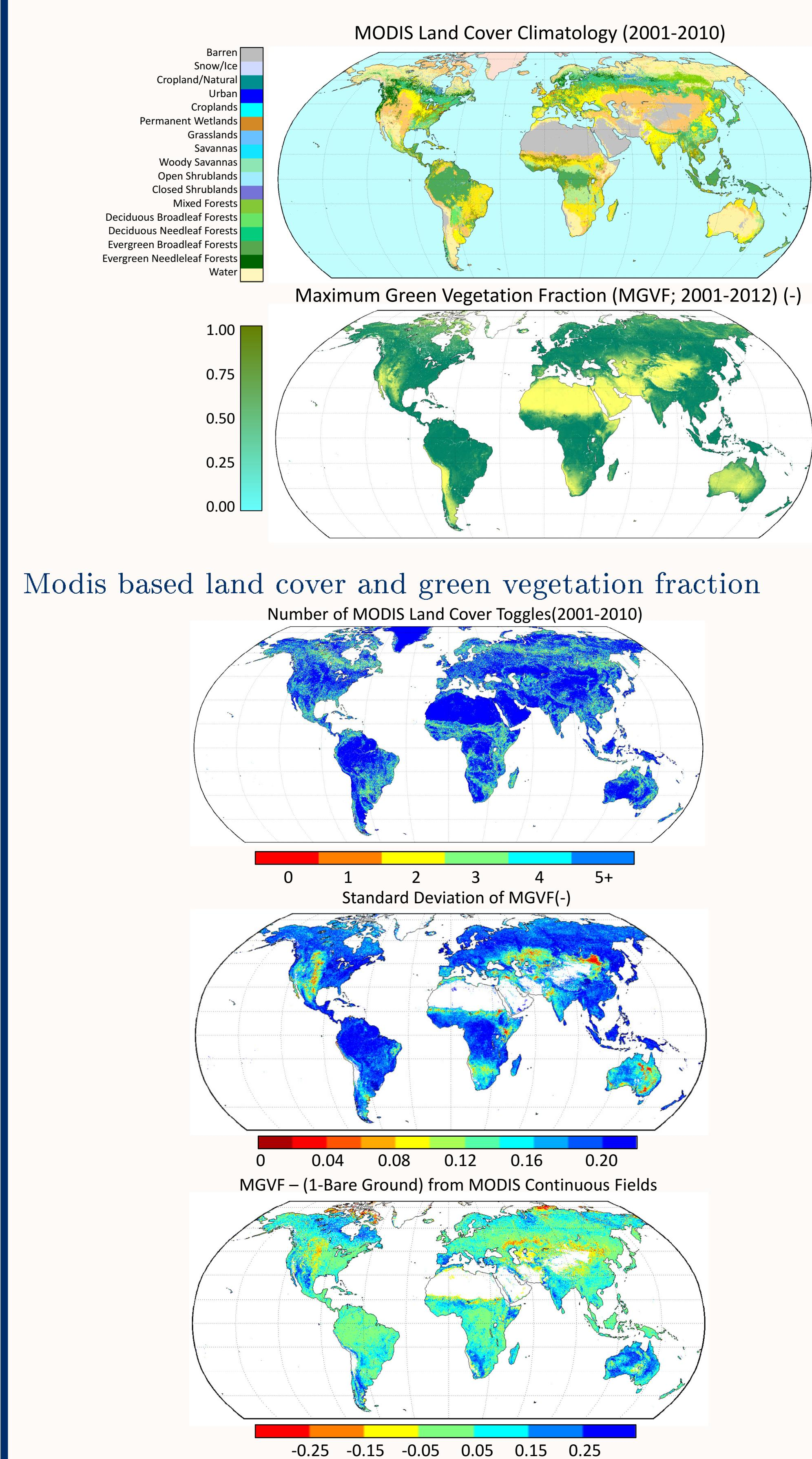
Toggling between different land cover types (top), the interannual variability of MGVF (middle), and comparison to the bare ground continuous fields (bottom)
