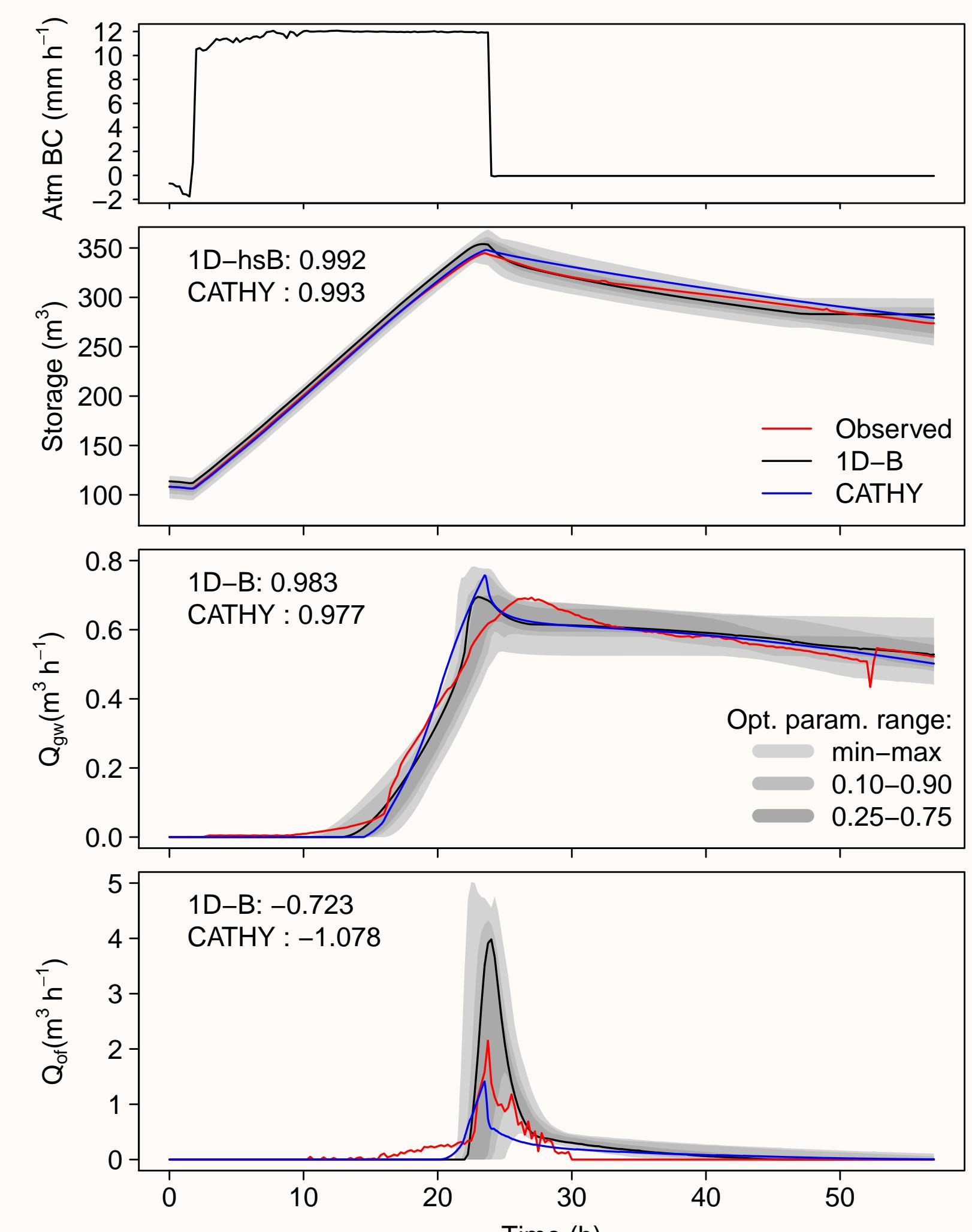
Observed and simulated storage and runoff behavior of hybrid 3-D approach and the 3-D Richards model CATHY
