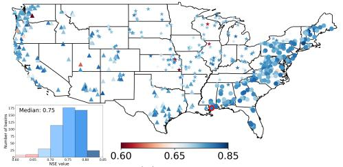
Our Geo-RS-LSTM model integrating remote sensing images, meteorological forcing sequences, and static catchment attributes accurately predicts streamflow at 531 basins across the CONUS.
