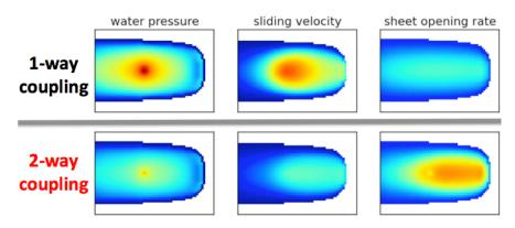
Model results demonstrating lower water pressure and sliding in the coupled hydrology/dynamics model due to increase of the basal water sheet capacity.
