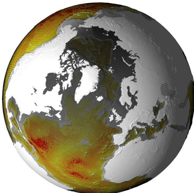
*A prototype is depicted for the E3SM arctic regionally refined ocean/sea ice grid with high resolution in the Arctic and North Atlantic Oceans.*
